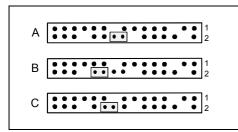
Pin pair A inserted = Skipping system and BIOS Setup password Pin pair B inserted =
